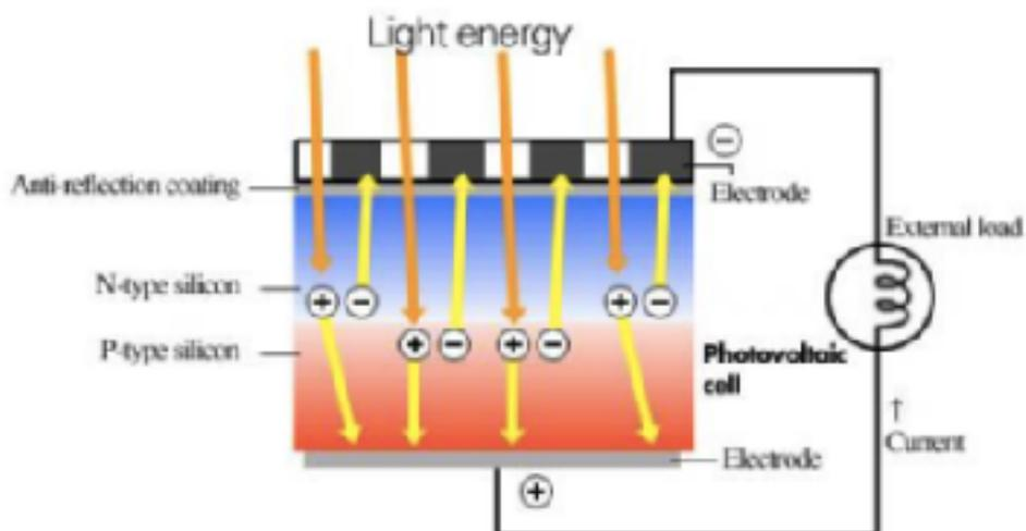
Figure 1: Basic Solar Cell Structure
