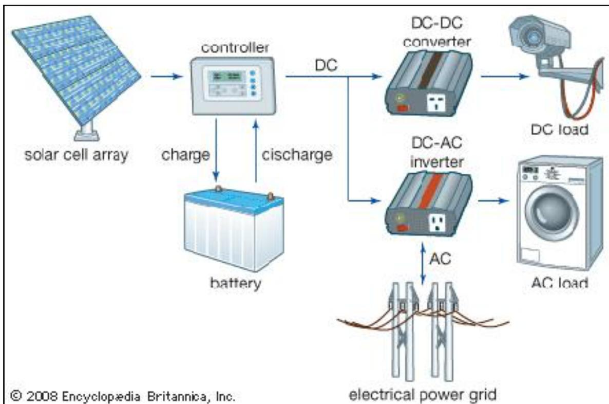
Figure 3: Typical solar power system diagram
